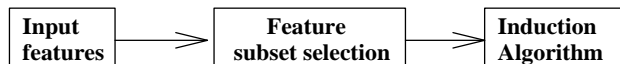
Figure 3: The feature filter model, in which the features are filtered independent of the induction algorithm.
