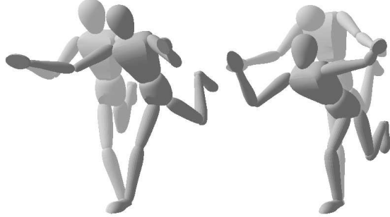
Figure 1. Comparison of configurations while performing a hand positioning task. By maintaining balance and maximizing mobility, the left humanoid has a markedly more natural posture than the one on the right.
