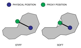
Figure 7: Physical Intuition Behind Stiffness Model
