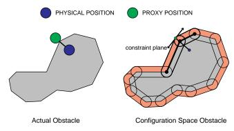
Figure 3: Configuration Space Obstacles & Constraint Planes
