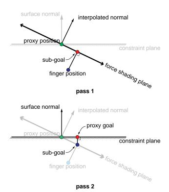
Figure 5: Two Pass Force Shading with Supplied Normals
