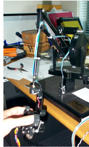
Figure 6. An asymmetric 6DOF haptic device that allows users to pinch virtual objects using index finger and thumb
