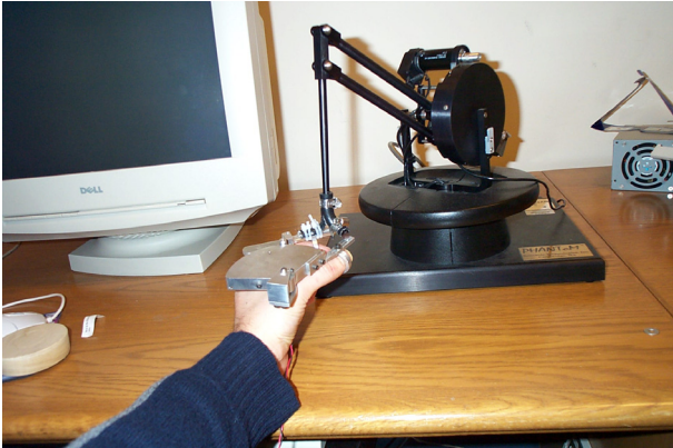
Figure 5. A four 4DOF haptic device that can be used for virtual grasping
