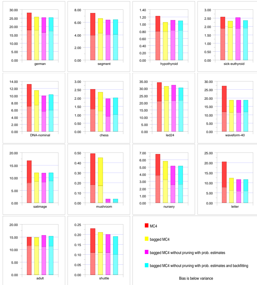
Figure 5. The bias-variance decomposition for MC4 and three versions of Bagging. In most cases, the reduction in error is due to a reduction in variance (e.g., waveform, letter, satimage, shuttle), but there are also examples of bias reduction when pruning is disabled (as in mushroom and letter).
