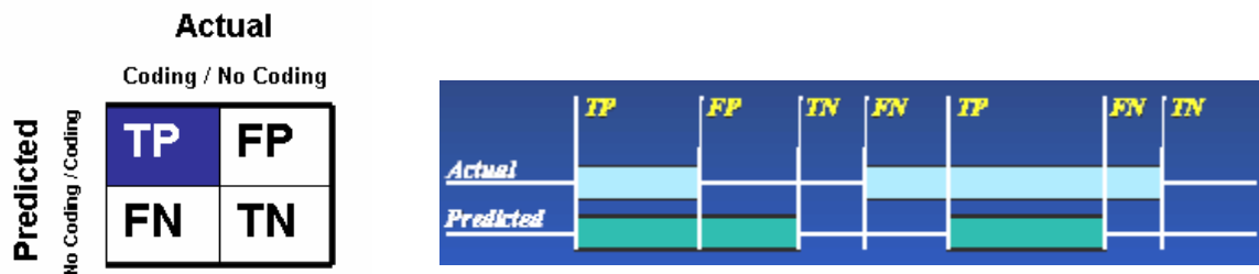
Figure 9: Summary of true positive (TP), false negative (FN), false positive (FP), and true negative (TN).
