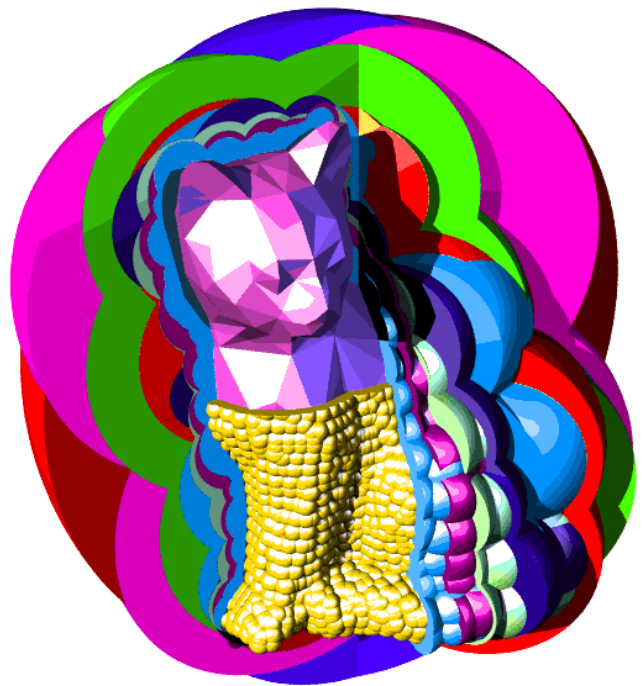
Figure 8: Cut-Away of the Bounding Hierarchy of a Cat Model
