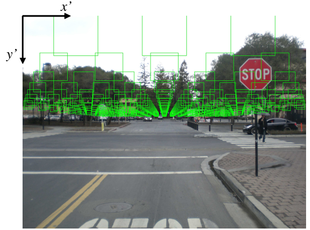
Figure 6: Projection of various possible 3D traffic sign locations into the 2D image plane using equation (2).
